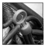
The dipstick is located toward the back of the engine compartment, next to the brake master cylinder. The dipstick handle is a bright red loop. See *Engine Compartment Overview on page 5-12* for more information on location.
